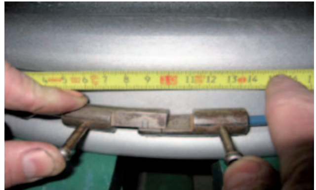
Mandrel gauge for rim circumference measurement
