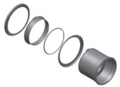
5-piece rim / all parts separate
